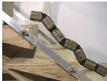
Fig. 7. Joint strength and stiffness: OT-4 lifting up three lead segments in order to reach the next step.
