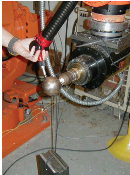
Fig. 15. Experiment Setup for robot stiffness measurement.
