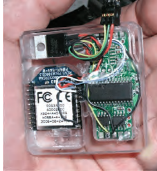
Fig. 25. Onboard components of the OT-4's wireless control communication system.
