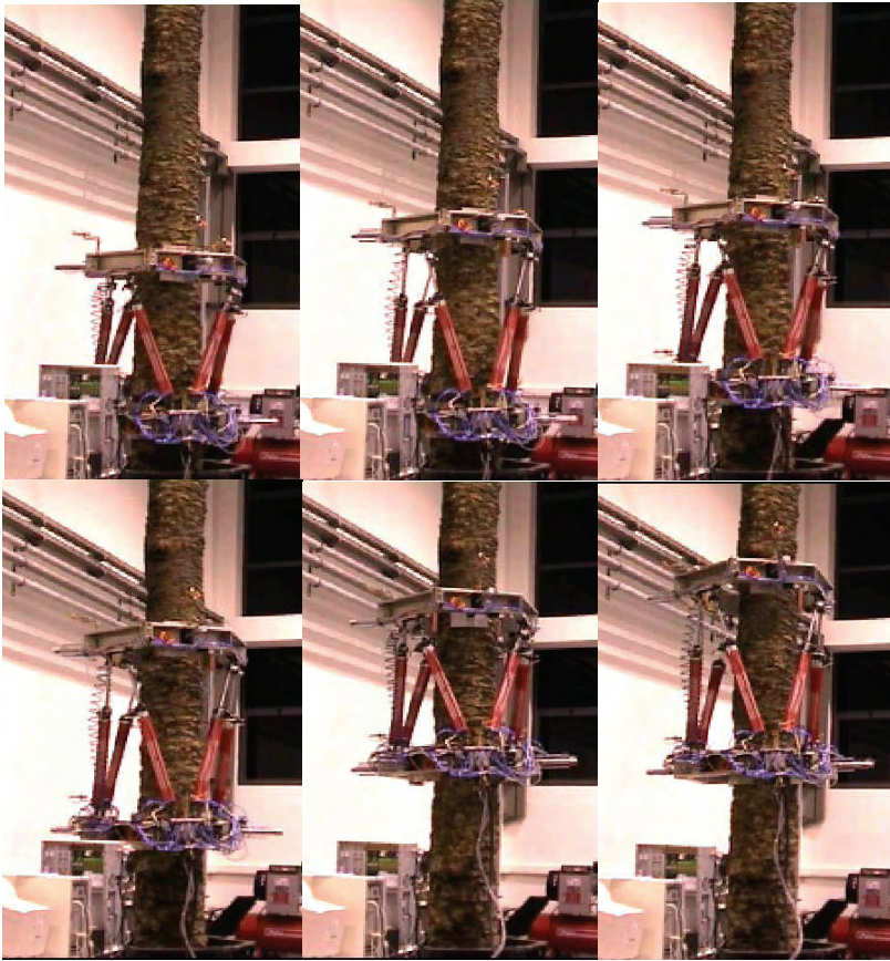
Fig. 5. Different images of the parallel robot climbing o a palm tree trunk.
