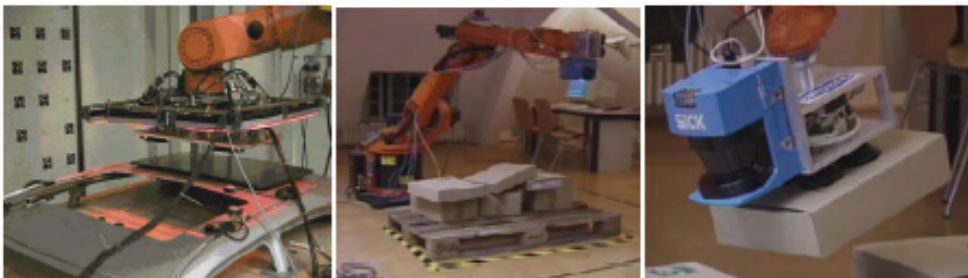
Fig. 10. (a) The sunroof fitting robot using four cameras in a closed loop control scheme and (b), (c) the depalletizing system during scanning and grasping
