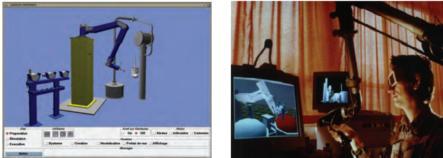
Fig. 4. TAO 2000 VR based telerobotic interface (CEA, France).
