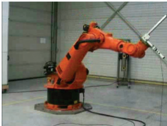
Fig. 9. Minimum of 3 LEDs are attached the tool frame during the calibration to obtain complete pose (6D). (Courtesy of Metris).
